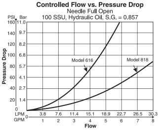
Controlled Flow vs. Pressure Drop Needle Full Open
